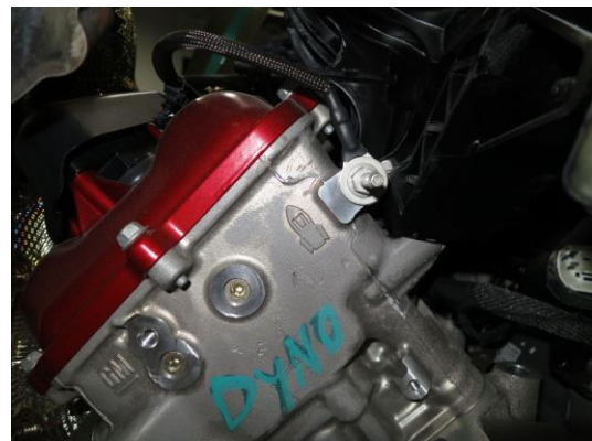
The NCM had just received this LT6 engine from GM. It was the engine that was run on a dynamometer for 8,000 continuous hours at varying speeds. The project
