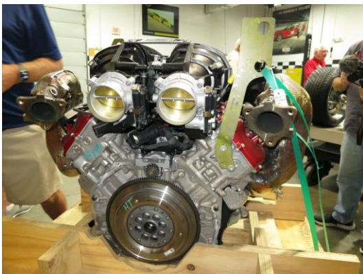
The NCM had just received this LT6 engine from GM. It was the engine that was run on a dynamometer for 8,000 continuous hours at varying speeds. The project
