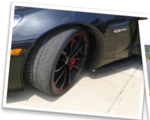
New tires and wheels for 2012. The Corvette team is opting for Michelin "Cup" tires, which are barely street-worthy racing slicks!
